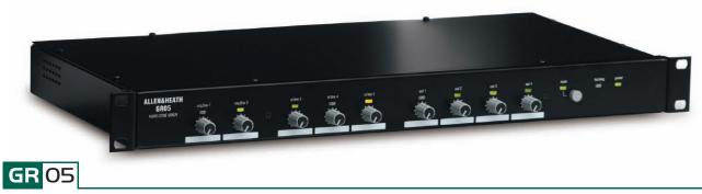
The GRO5 is a 5-input, 4-output analogue zone mixer for sound installations requiring 2 mic and 3 stereo line to up to 4 mono or 2 stereo zones. Internal jumpers allow custom configuration protected for day-to-day operation by non-technical staff. Zone volume may be remotely controlled.
